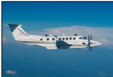
King Air aircraft have an operational range of 750 NM and provide 1 hour TOT
