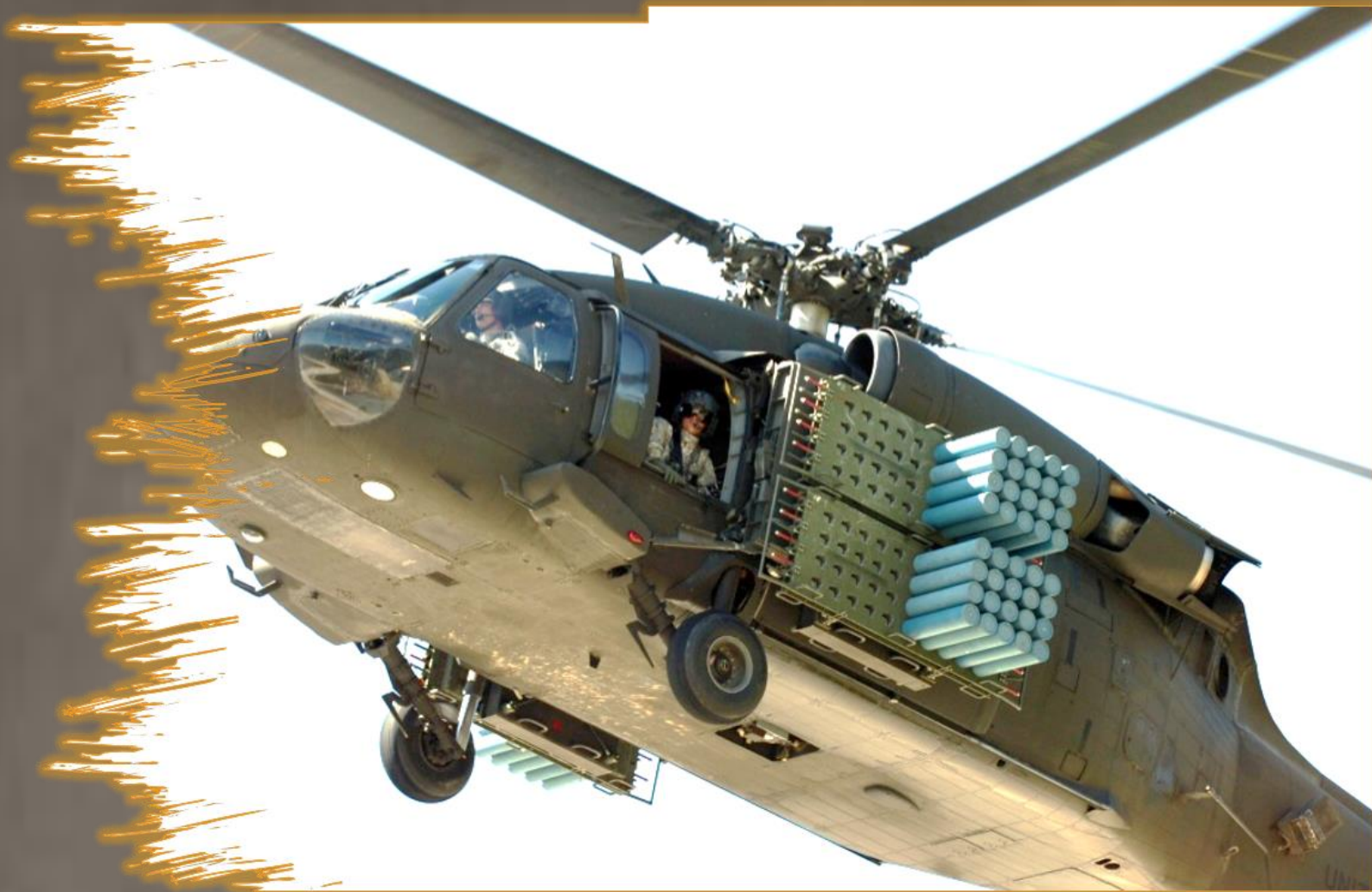
Soldiers from 2 nd Bn., 2 nd Aviation Regiment, 2 nd Combat Aviation Brigade, use a UH-60 Black Hawk helicopter to employ M-139 Air Volcano Mines. Photo courtesy of 2 nd CAB, Defense Visual Information Distribution System, Yangpyeong, South Korea.
