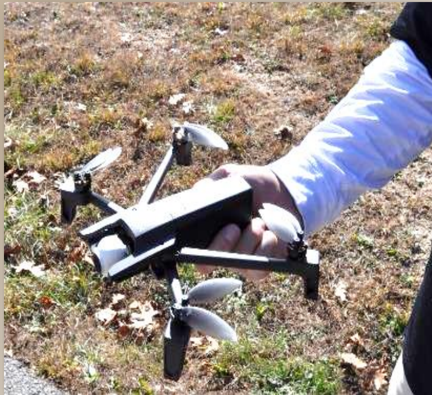
Photo Left: Devil's Elbow Trestle Bridge. Photo by Chief Baber. Photo top: COL Ken Frey, Matt Trani, and Casey Shanks with custom drone equipped with LiDAR. Photo by 1LT Matthew Hain. Photo bottom: Parrot Anafi drone for photogrammetric capture. This is COTS (commercial off the shelf) for $800. Photo by 1LT Matthew Hain. Photo right: LiDAR scan of the Devil's Elbow Trestle Bridge. Photo by SFC Andrew French & the NGA.
