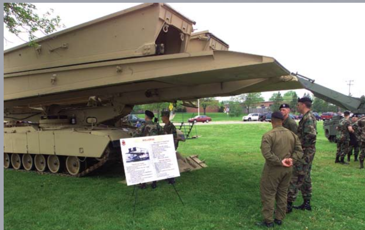
The Wolverine heavy assault bridge was in development for many years, and was designed in part to replace the 1960's era Armored Vehicular Assault Bridge (AVLB). The vehicle is shown here on display at the Engineer School in 2003. (Photo by FT Eyre)
